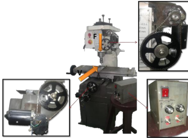
Figure 4. Drilling-Milling machine used for friction surfacing process
